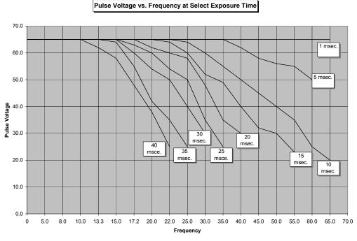
Figure #8 Pulse Voltage vs. Frequency
