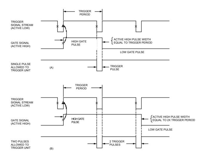
Figure #5 GATE Input Timing Diagram
