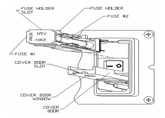
Figure #1 - AC Input Module
