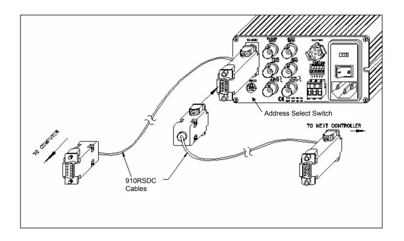
Figure #6 VMM-T1/D1 Daisy Chain Cable Configuration
