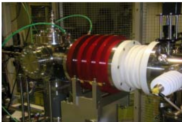
Fig. 5: Compact ECR ion source with permanent magnet.
