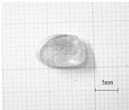
Fig. 7. A photograph of a  $\text{CaGa}_2\text{S}_4$  single crystal grown under excess sulfur. A cleaved surface is shown.
